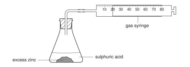
The same mass of zinc was used each time. The volume of acid used was different each time. Use the syringe diagrams to record the volume of hydrogen produced each time in the table.
